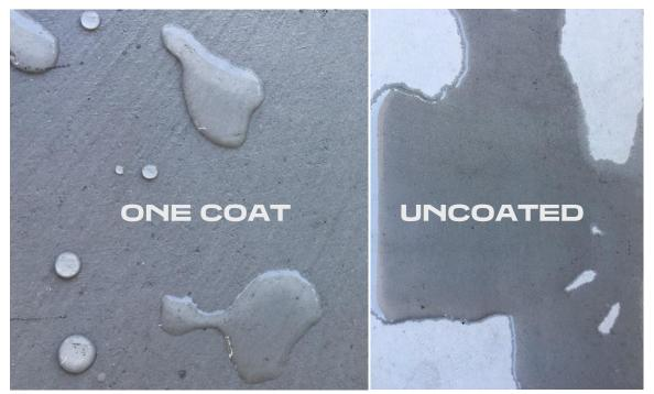
**Description:** A waterbase, 2-in-1 hybrid sealer that uniquely both penetrates and seals. Product will increase water repellency, block micro-organism growth, and seal any chips or scratches. *Repelz Penetrating Silane Siloxane Concrete Sealer* will not change colors or efflorescence over time.
